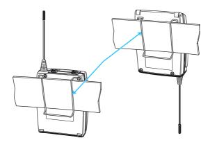
The clip is detachable so that you can also attach the receiver with the antenna pointing downwards. To do so, withdraw the clip from its fixing points and attach it the other way round.
